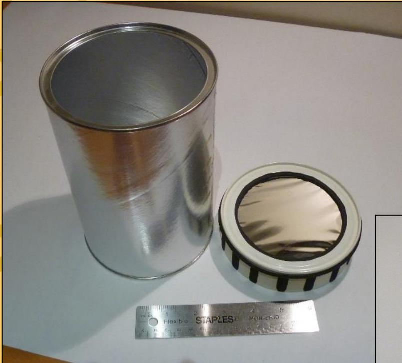
**4in (100mm) Solar Filter with Baader AstroSolar Safety film**
